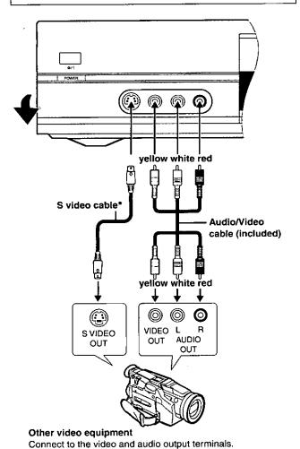
Connecting to the input terminals on the rear of the unit, L1 and L3
